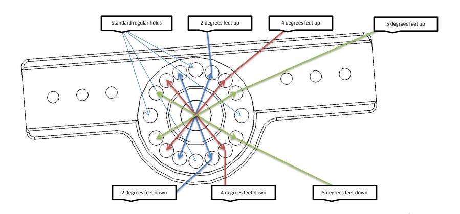
• The foot swivel can be rotated 11.25 degrees or 22.5 degrees downward. This starts another set of standard regular holes in which all of the 4 starting positions and the 7 incremental positions repeat themselves.
