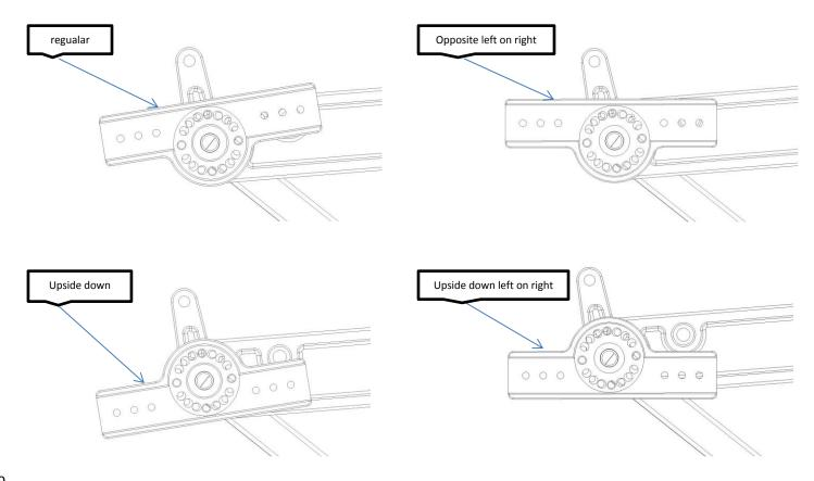
• The foot swivel has many possible incremental angles within each above mentioned starting position. To adjust foot swivel incremental angles, remove the foot rest assembly. Remove the foot swivel bolts and loosen main foot swivel bolt. Rotate foot swivels to desired position, replace all bolts and tighten. Replace foot rest assembly and all associated bolts and tighten.
