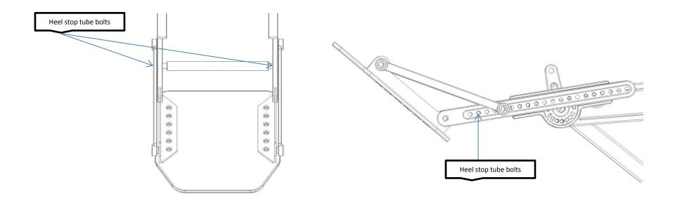
• If the heel stop tube's desired position is between the foot swivels, the spacers in the ends of the tube need to be removed.
