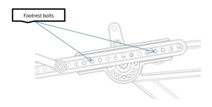
• Remove the supplied bolts and angle the footrest to desired angle. Replace the bolts and tighten. Positioning and adjustment is rider's preference. (page10-13)
