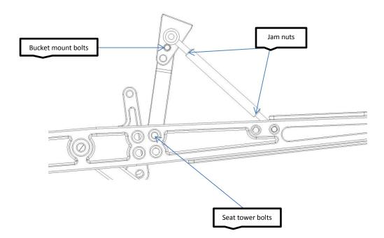
• The bucket mount can also be moved up or down to achieve the height desired. To move bucket mount up or down remove the bucket mount bolts and the upper seat tie rod bolts and place bucket mount in desired position. Upper tie rod bolts must be removed first (there is a spacer behind upper seat tie rod that must be replaced in any of the 3 positions.)
