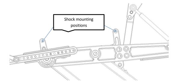
• Pull the shock tower back. Remove the seat cross member bolts from the seat cross member. Install those bolts through the red rod ends and into the supplied cross member on the inside of the frame and tighten. Positioning and adjustment is the rider's preference. (page 7-8)
