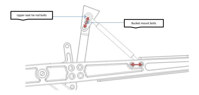
• The bucket mount can be placed in any of the 3 positions available on the seat tower. Inorder to achieve a leveraged triagulation the seat tie rod must be in a different hole than the bucket mount bolts, this allows the seat tower and bucket mount angles to change indepedently with the lengthening or shortening of the seat tie rods.
